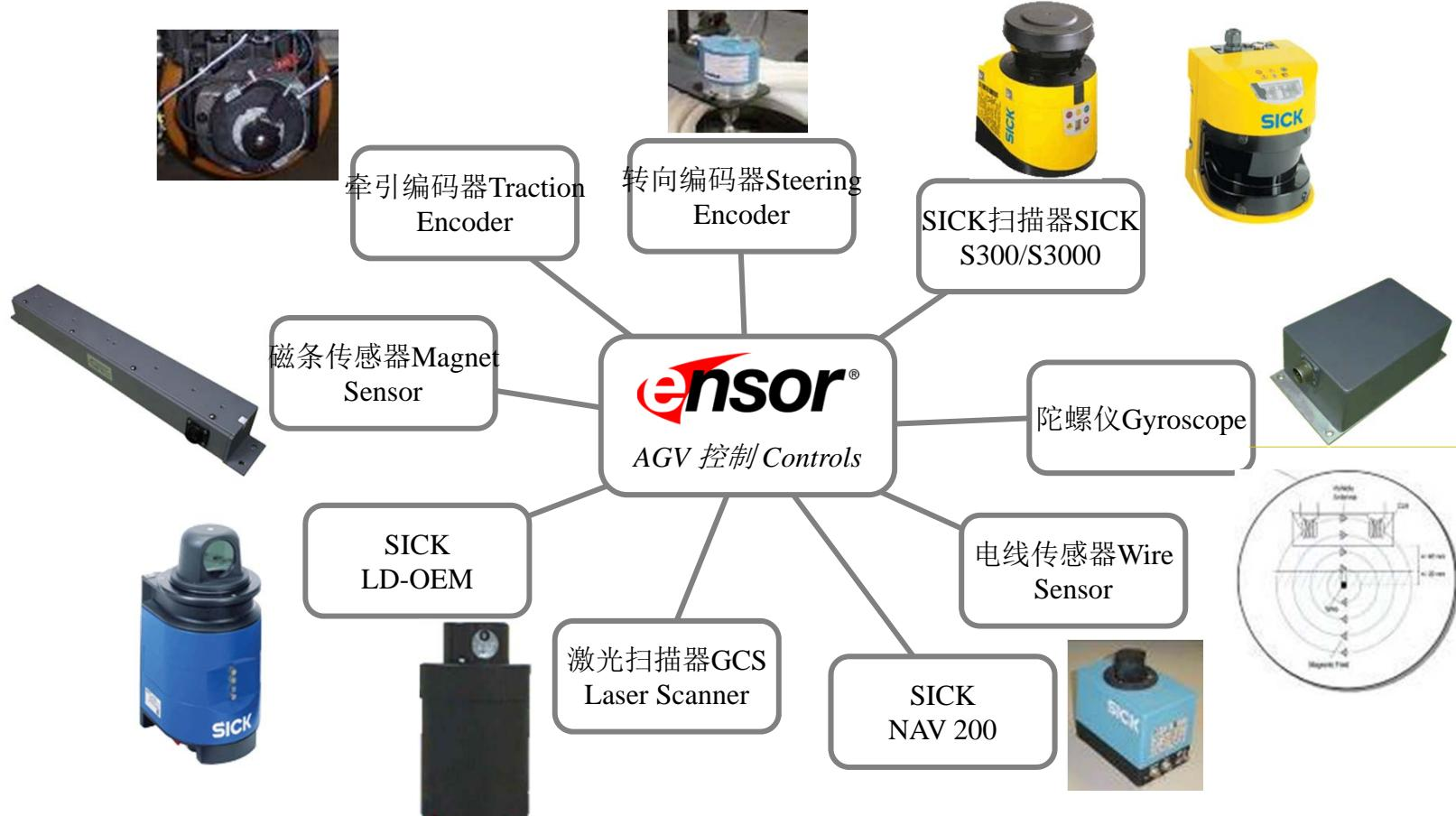
所有合适的导航传感器都被不停使用 All navigation capable sensors are continuously used
